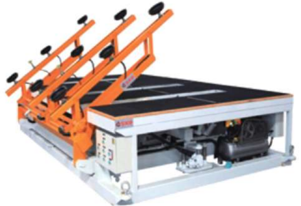
Multi Functional Manual Cutting Table with Air Cushion & Breaking Bars
